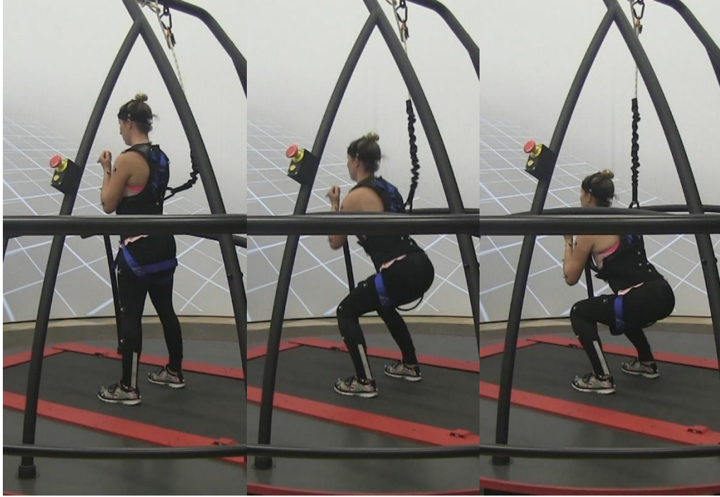
Figure 21: Stages of Squat Exercise with Dynamic Platform in Heave Condition
